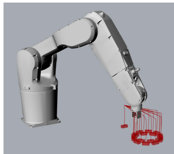
Figure 1: Robotstudio simulation performing scripted pick-and-place tasks
