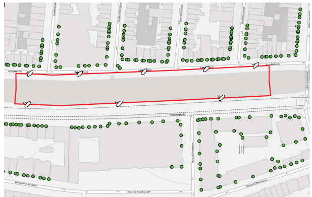
Figure 4: Impression of the number of precise levelling points around the Boerenwetering garage
