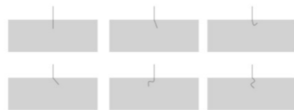
Figure 1: Six examples of fiber orientation at a crack interface.
