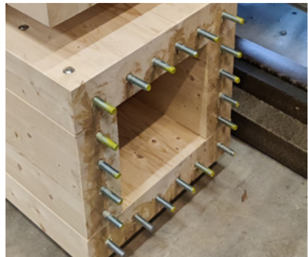
Figure 3: Cross-section with glued-in rods
