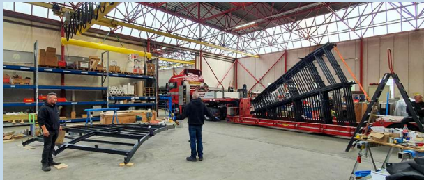
Figure 1: Roof segments in the factory (Photo: Octatube)
