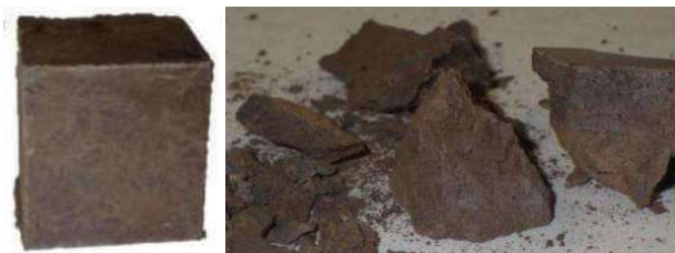
Figure 3: Cube specimen (a) before and (b) after unconfined compression test
