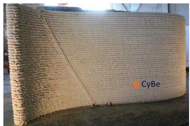
Figure 3: 3D printed curved concrete wall by CyBe
