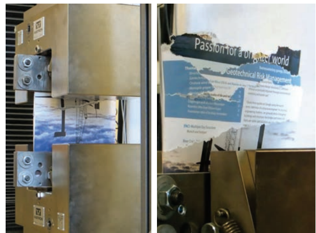
Figure 2: Test setup and result of tensile test
