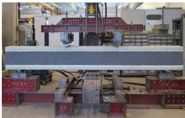
Figure 3: Four-point bending test on a sandwich beam with reinforced faces and an EPS core
