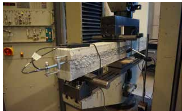
Figure 2: Four-point bending test on a sandwich beam with an ultra-lightweight concrete core
