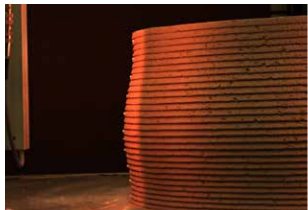
Figure 3: Instability failure during the printing process
