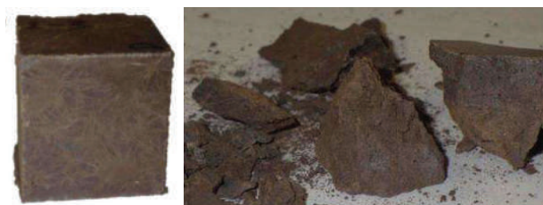
Figure 3: Cube specimen (a) before and (b) after unconfined compression test
