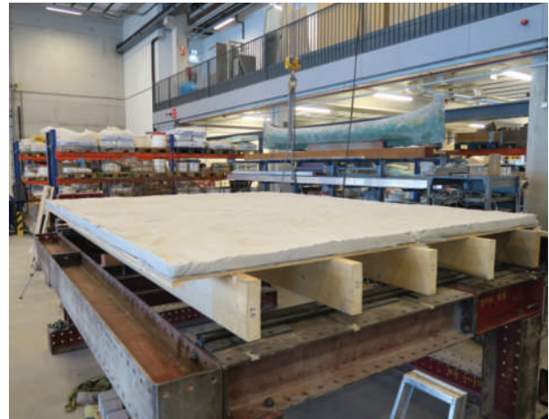
Figure 1: Timber concrete floor used for the experimental tests
