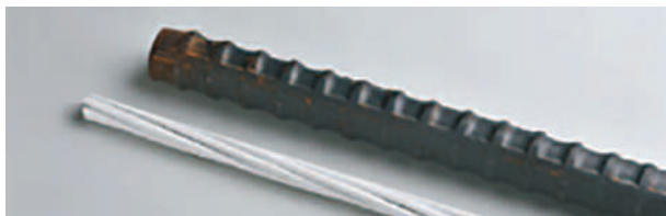
Figure 2: Carbon fiber compared to conventional reinforcement
