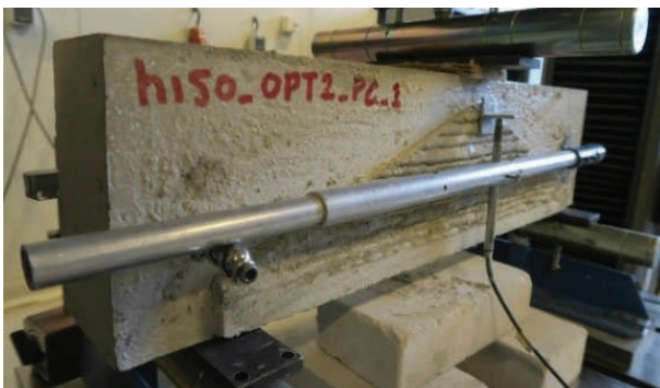
Figure 4: Slender beam optimized by functional grading (h150_OPT2)
