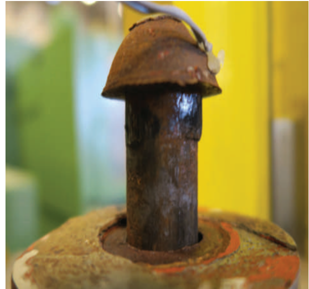
Figure 2: The instrumented specimen used to measure the residual clamping (axial) residual force in the rivet. A special strain gauge is inserted in a hole produced in the shaft of the rivet, while it is clamping the plates. Subsequently, the rivet is ejected and the value of the initial clamping force is determined by measuring the relaxation of the rivet. The picture refers to a test terminated.
