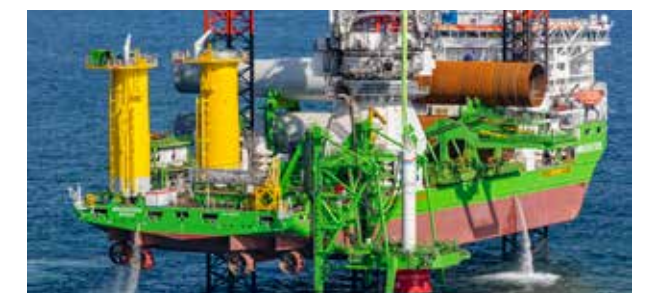
Figure 2: TWD's gripper design on DEMA's vessel Innovation
