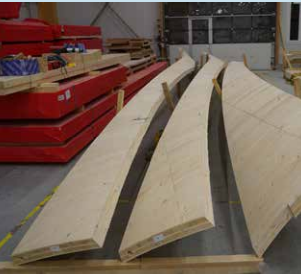
Figure 2: Curved CLT panels in final, form stable form
