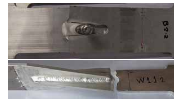
Figure 3: Failed specimens (bearing failure and longitudinally welded variant 1)
